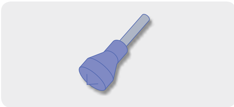
Figure 11: Image of probe-tip illustrating a nipple-tip extrusion
