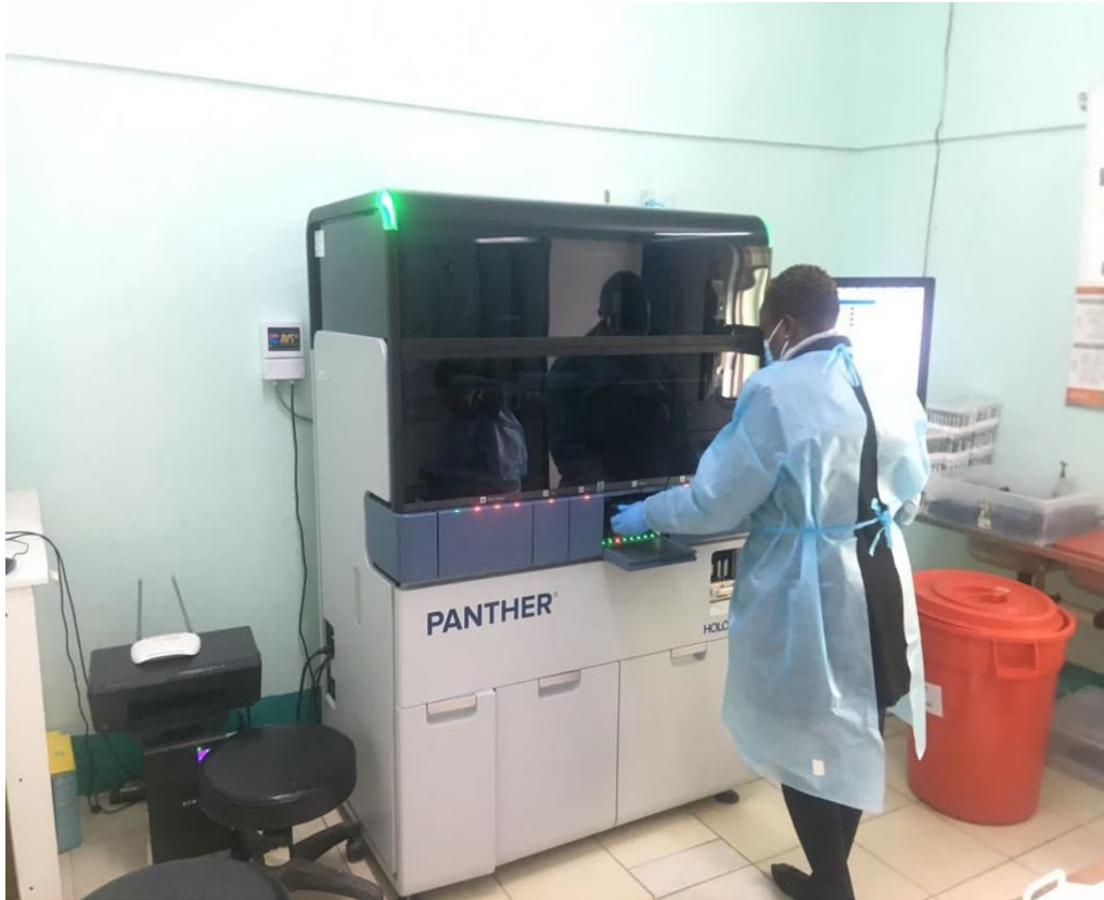
Zimbabwe – HPV testing being carried out on the Hologic Panther machine at Marondera Laboratory
